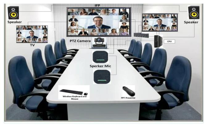
The following are the key components of the Smart VC setup for training: Desktop Computer (AIO) – Core i7 System for IP based VC Video Conferencing System: Camera & Expansion Mic.
